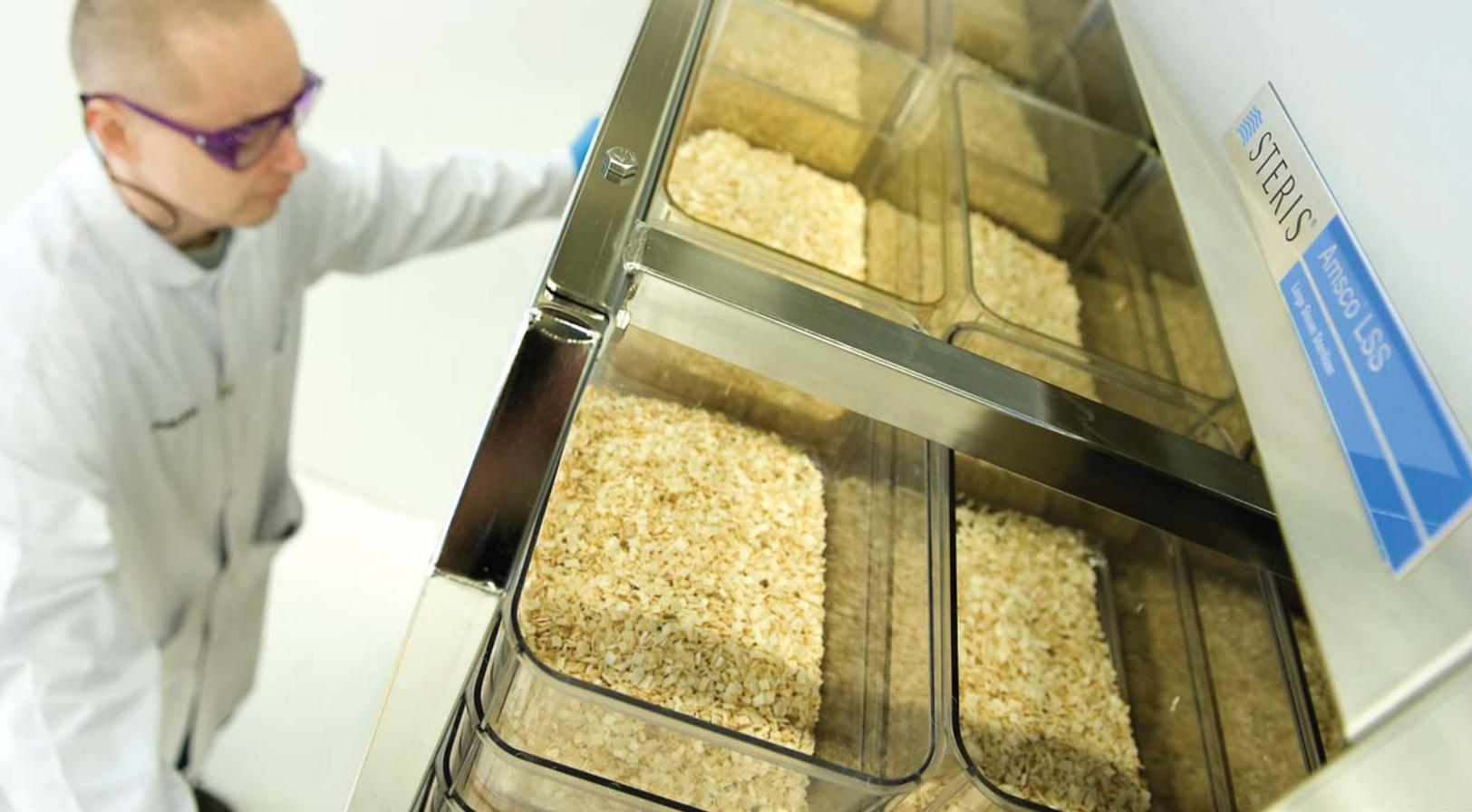
The AMSCO LSS Sterilizer is designed to process laboratory animal caging systems and associated equipment. The LSS incorporates several features to maximize productivity, provide flexibility, and ensure safety and reliability. The LSS was also developed with the sustainable laboratory in mind.
